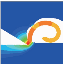
New tooth design with chip breaker
